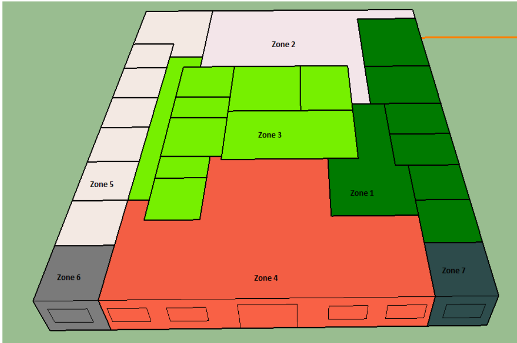
Figure 41. Seven thermal zones air-conditioned by four GEHP units
